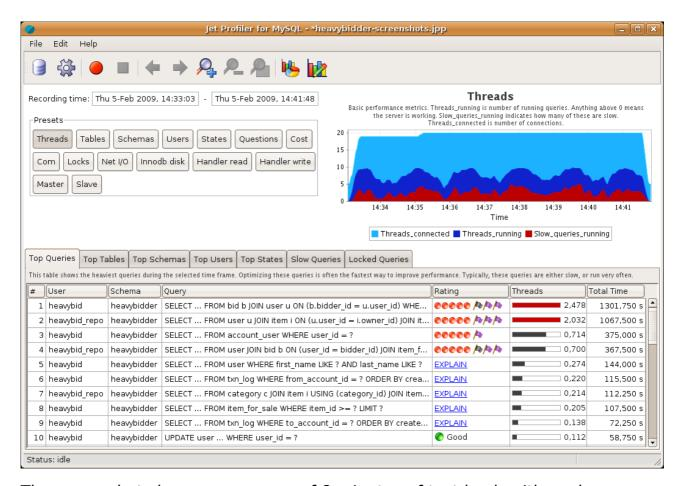
The screenshot shows a sequence of 8 minutes of test load, with peaks every 90 seconds. The Top Queries table shows which queries are most frequently observed along with a rating based on EXPLAIN. This view is the most important tool to find the worst performing queries.
